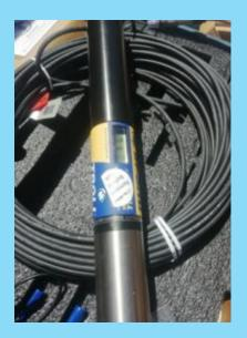
The electrical conductivity of the first well is 2000 us/cm and of the second well is 6740 us/cm. The two chosen wells for the installation of a multiparameter sonde for the real-time monitoring of groundwater are used mainly for irrigation.
